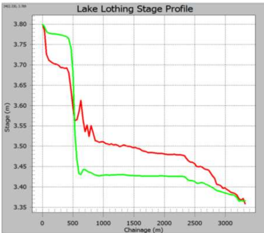
Figure 13 Head loss through Bascule Bridge for the 1 in 1000yr event from the coast to Mutford Lock (original ISIS 2D model is red, revised Tuflow version is green)
